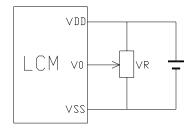
V<sub>DD~</sub>V<sub>0</sub>: LCD Driving voltage
