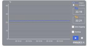
$\diamondsuit$  Data logging: All temperature data is saved as a text file in a subfolder "TEMPLOG". Logging can be started and stopped manually.
