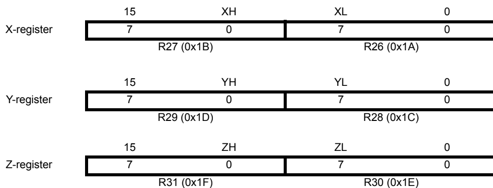
Figure 3-3. The X-, Y-, and Z-registers
