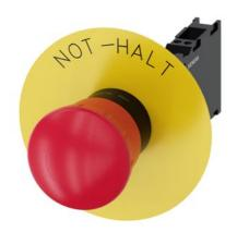
EMERGENCY STOP mushroom-type actuator, 22 mm, round, plastic, red, 40 mm, positive latching, according to EN ISO 13850, rotate-to-unlatch, with yellow backing plate, inscription: NOT-HALT, with holder, 1 NO+1 NC, spring-type terminal, Z=20-unit packaging
