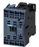
Contactor, AC-1, 50 A/400 V/40  $^\circ\text{C},$  S0, 4-pole, 125 V DC, 1 NO+1 NC, Spring-type terminal
