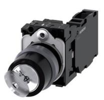
RONIS key-operated switch, 22 mm, round, plastic with metal front ring, lock number SB30, with 2 keys, 2 switch positions O-I, latching, actuating angle 90°, 10:30h/13:30h, key removal O+I, with holder, 1 NO+1 NC, screw terminal, Z=20-unit packaging
