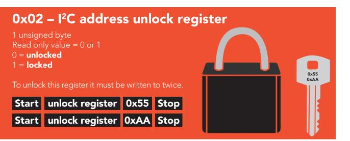
The two unlock commands must be sent back to back in immediate succession. No other write, or read event can occur. Once the register is unlocked it will equal 0x00 (unlocked).
