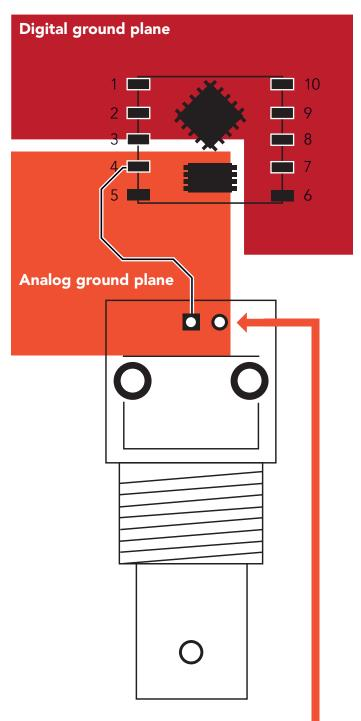
Connect pin 2 on the BNC/SMA to the analog ground plane
