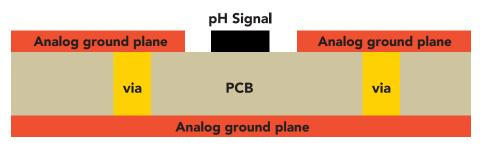
This cross section is an example of how the analog ground plane protects the pH signal. The analog ground should surround the pH signal, on both the top and bottom layers.
