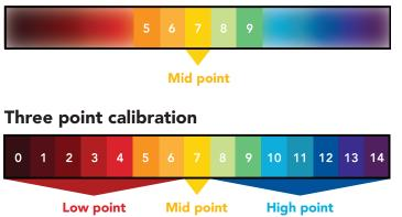
Three point calibration will provide high accuracy over the full pH range. Three point calibration at **4.00**, **7.00** and **10.00** should be considered the standard.
