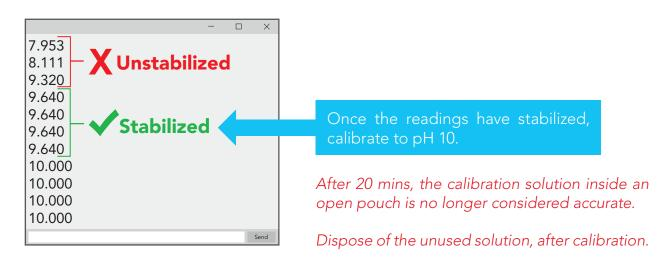
The pH OEM<sup>m</sup> circuits default temperature compensation is set to 25° C. If the temperature of the calibration solution is +/- 2° C from 25° C, consider setting the temperature compensation first. **Temperature changes of < 2° C are insignificant.**
