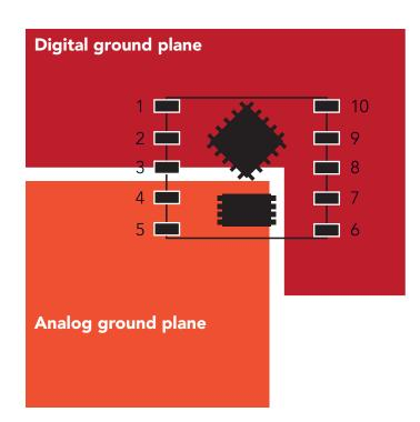
2 Connect pin 5 to the analog ground plane, and pin 6 to the digital ground plane.
