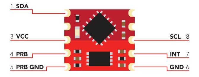
The pH OEM<sup>™</sup> circuit requires two separate ground planes to operate properly. One ground plane is for the digital section of the device, the other is for the analog section.
