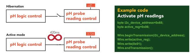
Once the device has been woken up it will continuously take readings every 420ms. Waking the device is the only way to take a reading. Hibernating the device is the only way to stop taking readings.
