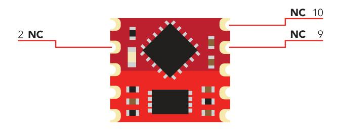
7 If the pH OEM<sup>™</sup> circuit is going to be hand soldered, avoid using rosin core solder. Use as little flux as possible. Do not let liquid flux seep under the pH OEM<sup>™</sup> circuit. After the pH OEM<sup>™</sup> circuit has been soldered to the PCB all flux residue *MUST* be removed. Failure to do so will result in poor quality readings.
