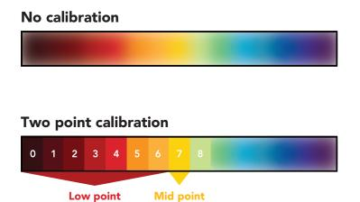
Two point calibration will provide high accuracy between 7.00 and the second point calibrated against, such as a **4.00**.
