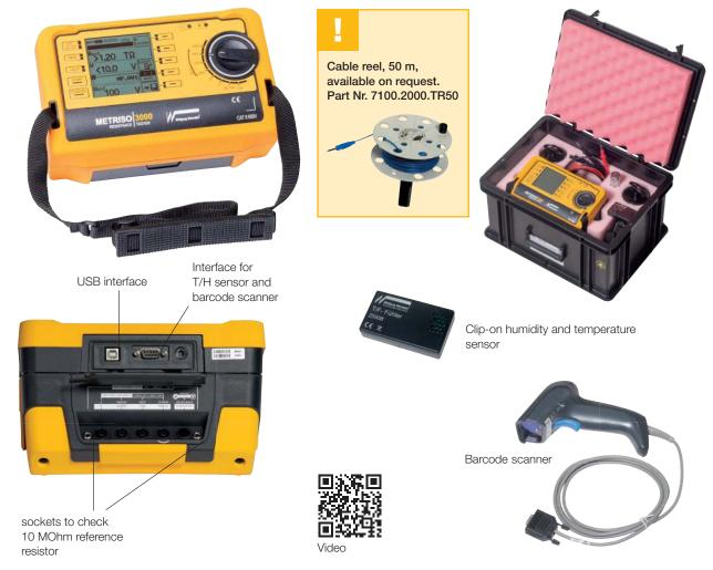
Metriso<sup>®</sup> 3000 - test kit includes: digital high resistance tester, temperature and relative humidity sensor, USB port, PC software ETC for Windows<sup>®</sup>, 2 probes, a hand-held probe with connecting cable, user's instructions in German, English and French, calibration certificate, conductive carrying case fitted with dissipative pink foam.
