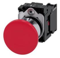
Mushroom pushbutton, 22 mm, round, metal, shiny, red, 40mm, latching, pull-to-unlatch mechanism, with holder, 1 NC, screw terminal, with laser labeling, inscription or symbol Customer-specific selection with SIRIUS ACT configurator (CIN)
