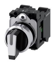
Selector switch, illuminable, 22 mm, round, metal, shiny, white, selector switch, short, 3 switch positions I>O<II, momentary contact type, actuating angle 2x45°, 10:30h/12h/13:30h, with holder, 1 NO, 1 NO, Spring-type terminal
