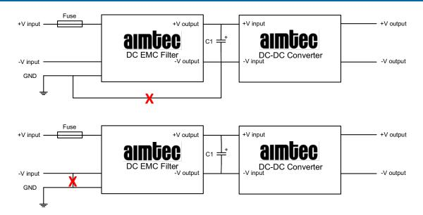
Note: Connections marked with X interfere with this filter modules performance and should therefore not be used
