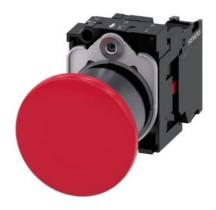
Mushroom pushbutton, 22 mm, round, plastic with metal front ring, red, 40mm, latching, pull-to-unlatch mechanism, with holder, 1 NC, screw terminal, with laser labeling, inscription or symbol Customer-specific selection with SIRIUS ACT configurator (CIN)
