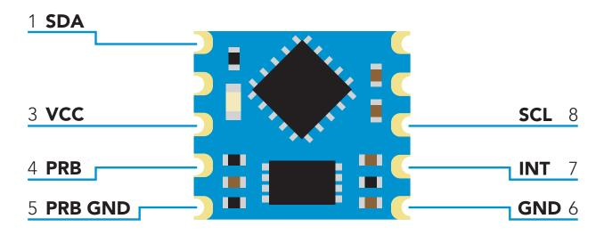
The ORP OEM<sup>™</sup> circuit requires two separate ground planes to operate properly. One ground plane is for the digital section of the device, the other is for the analog section.
