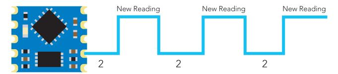
The pin will not auto reset. 2 must be after each transition from low to high.
