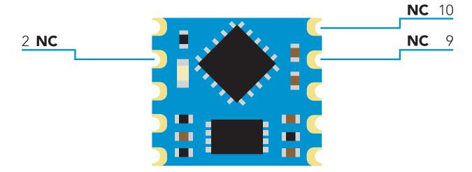
If the ORP OEM™ circuit is going to be hand soldered, avoid using rosin core solder. Use as little flux as possible. Do not let liquid flux seep under the ORP OEM™ circuit. After the ORP OEM™ circuit has been soldered to the PCB all flux residue MUST be removed. Failure to do so will result in poor quality readings.
