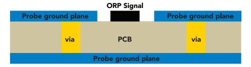
This cross section is an example of how the analog ground plane protects the ORP signal. The analog ground should surround the ORP signal, on both the top and bottom layers.
