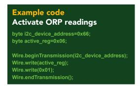
Once the device has been woken up it will continuously take readings every 420ms. Waking the device is the only way to take a reading. Hibernating the device is the only way to stop taking readings.
