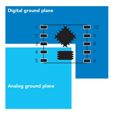
Connect pin 5 to the analog ground plane, and pin 6 to the digital ground plane.
