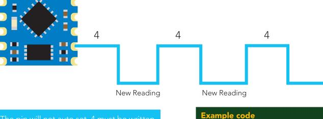
The pin will not auto set. 4 must be written to the interrupt control register after each
