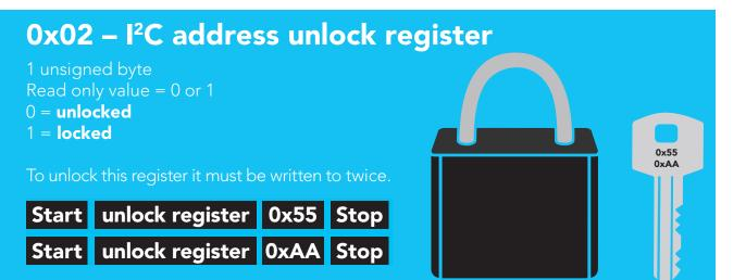
The two unlock commands must be sent back to back in immediate succession. No other write, or read event can occur. Once the register is unlocked it will equal 0x00 (unlocked).
