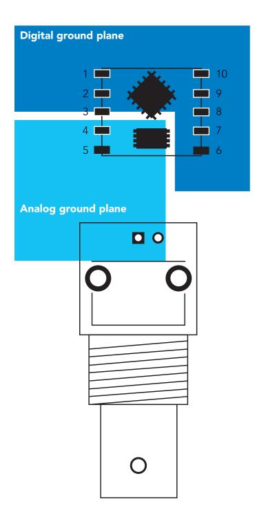
Using a 0.4mm trace width connect pin 4 (PRB) to pin 1 on the BNC/SMA. Keep this trace as short as possible. This trace is the ORP signal path.
