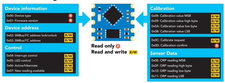
The default device address is **0x66** This address can be changed.
