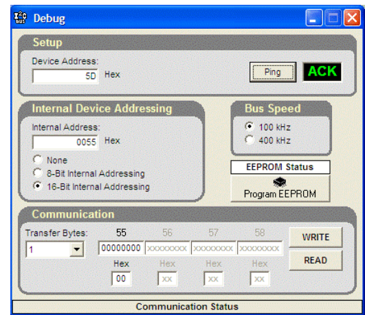
Figure 29. Evaluation Software I 2 C Debug Window
