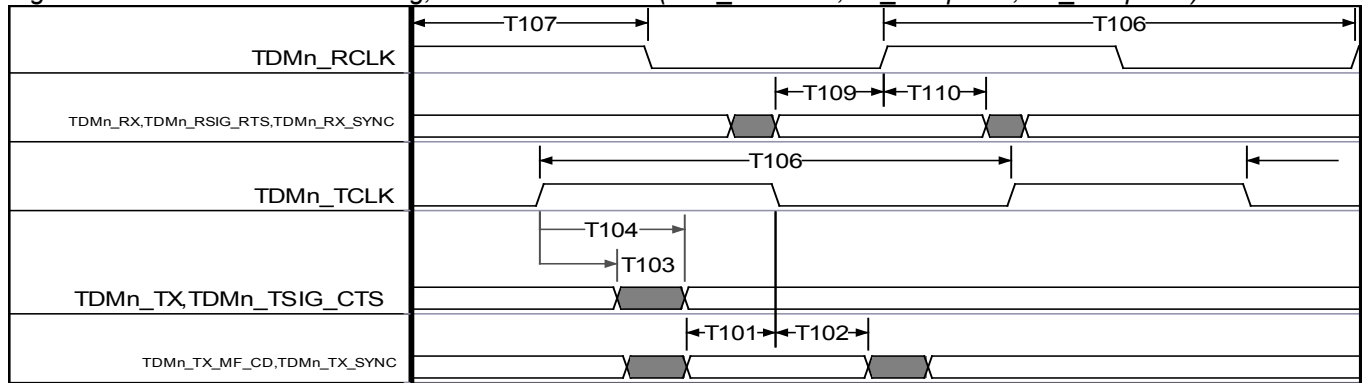
Figure 14-12. TDMoP TDM Timing, Two Clocks Mode (Two_clocks=1, Tx_sample=0, Rx_sample=1)
