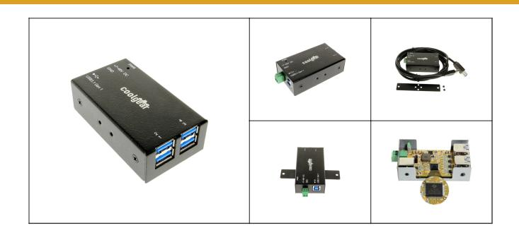
Built with industrial environments in mind, the 4 port, 7-48V DC variable voltage, USB 3.1 micro hub is a compact solution. Compliant with USB 3.1 specifications, the hub has data speed up to 5GBps. It includes a surface mounting kit but can be mounted on a DIN Rail.
