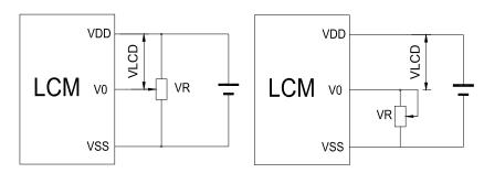
VDD~V0: LCD Driving voltage
